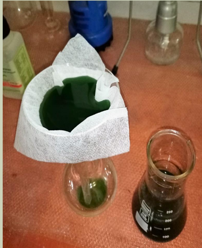
Fig.3.6 Washing Spirulina with 1g/l solution of NaCl
